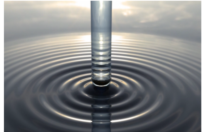
This computer rendering illustrates the results of a simulation studying a ripple phenomenon in a water jet caused by surface tension.
